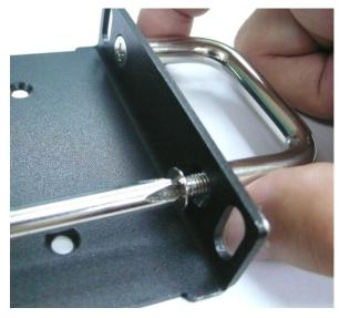
Step 3: Installing the rack ears to the DA-685
