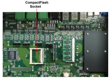
${\tt 3.} \quad \text{Insert the CompactFlash card into the socket. Push downwards to make sure that the card is firmly inserted.}$
