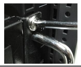
**NOTE** Four screws are required to attach the DA-685 to the rack. Use two screws on the left side and two screws on the right side.
