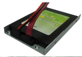
Place the drive bracket into the mounting space; fasten the bracket to the case using four screws, one on each corner
