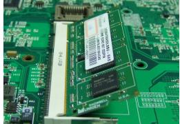
6. Push the memory all the way down to complete installation.
