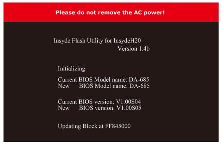
6. Once the upgrade is finished, the computer will automatically reboot. To check and see if the upgrade was successful, navigate to the **BIOS Main Page** and note the **BIOS Version number**.
