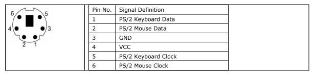
Use the Y-type cable to convert the mini-DIN connector into two 6-pin mini-DIN connectors to connect both a PS/2 keyboard and PS/2 mouse at the same time. (The Y-type cable is not included in the accessory package. It should be purchased separately. You may also use the USB ports to connect your USB-based keyboard and mouse.)
