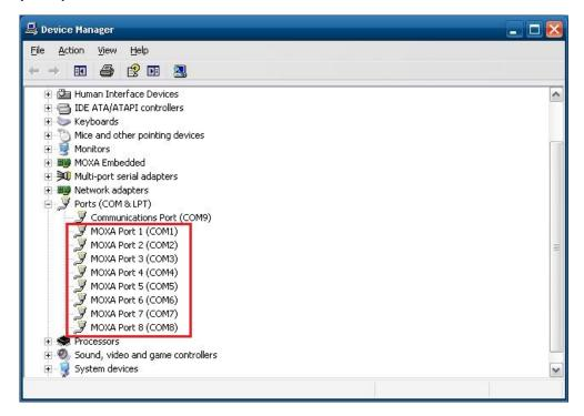
The Port 1 and Port 2 are RS-232/422/485 serial ports. Right-click the **COM** port you wish to configure, and then select **Properties**. Select **Port Settings** tab for further configuration. Note that they support bit rates up to **115,200** bps. Click **OK** to finish.
