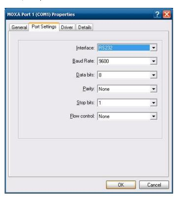
Ports 3 to 8 are 2-wire RS-485 terminal blocks. Right-click the **COM** port you wish to configure, and then select **Properties**. Select **Port Settings** tab for further configuration. Note that they support the bit rates up to **115,200** bps. Click **OK** to finish.
