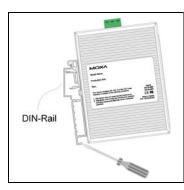
To remove Moxa EDS-205 from the DIN-Rail, insert a flat-blade screw driver horizontally into the DIN-Rail kit under the EDS-205, and then pull it upwards and release the EDS towards you and away from the DIN-Rail
