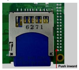
**Step 4:** Before using the SD card, check the /etc/rc file to ensure that the driver module for the SD card control is loaded. The loading sequence should be as follows:
