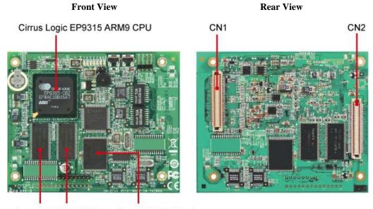
onboard 128 MB RAM onboard 32 MB Flash EM-2260-DK Carrier Board and Peripheral Extension Board
