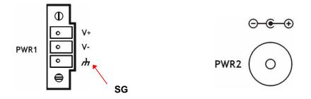
The Shielded Ground (SG, sometimes called Protected Ground) helps to limit the effects of noise due to electromagnetic interference (EMI). Run the ground connection from the ground screw to the grounding surface prior to connecting devices.
