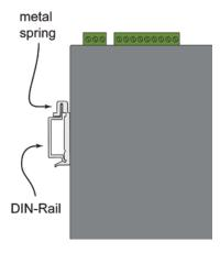
To remove the IA240 from the DIN-Rail, simply reverse Steps 1 and 2.
