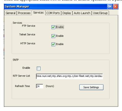
You can also use SNTP to adjust the time automatically. To do this, check mark the **Enable** check box under SNTP, and then click **Save Settings**.
