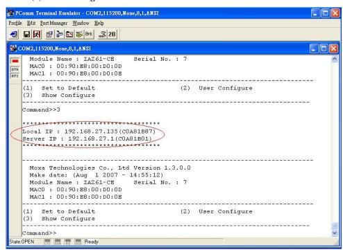
After confirming the IP configuration, press ESC to return to the main menu.
