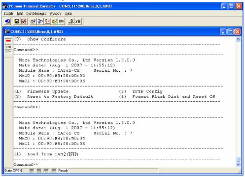
Select (1) Load from LAN2 and then input the firmware file name (e.g., IA260CE\_V1.0\_0704210.hfm) and press Enter.
