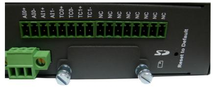
3. Be sure to insert the SD card correctly into the protective cover, as shown in the figure below. Push inward and make sure that the SD card has been completely plugged in.
