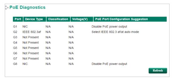
**PoE Diagnose** helps users determine the PD conditions. The system provides the user with configuration options; select the best option for your PDs. Take the following steps to diagnose PD conditions:
