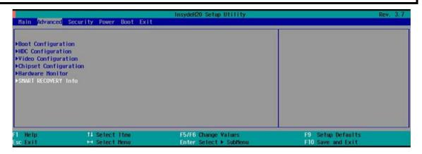
3. Use the up/down arrows to navigate to **SMART RECOVERY Info** and press **Enter** to open Smart Recovery's BIOS setup page.
