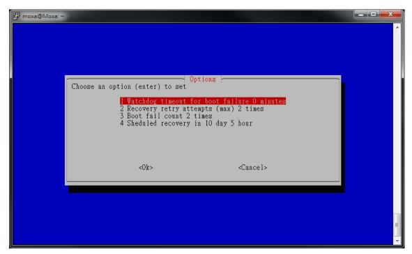
1 Watchdog timeout for boot failure...: If your system OS does not boot successfully within the timeout minutes specified here, the system will reboot automatically. The range is 0-255. The value 0 is used to disable the watchdog timeout.
