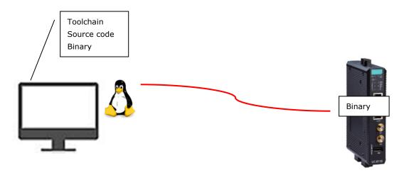
To ensure that an application will be able to run correctly when installed on the UC-8100-LX, you must ensure that it is compiled and linked to the same libraries that will be present on the UC-8100-LX computer. This is particularly true when the RISC Cortex processor architecture of the UC-8100 differs from the CISC  $\times$ 86 processor architecture of the host system, but it is also true if the processor architecture is the same.
