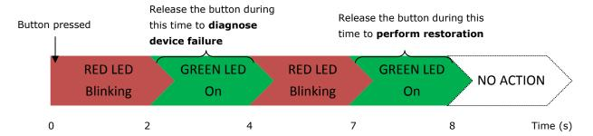
The LED indicators have different behaviors when diagnosing for device failure and for performing firmware restoration as listed in the table below:
