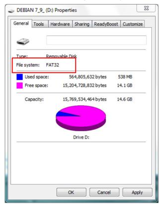
4. If the SD card is not using a FAT32 file system, you will need to format it to a FAT32 file system.
