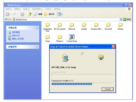
4. Double-click on the CAB file to start installing the UPort 1100 series WinCE driver. After installing the driver, plug the UPort 1100 series device into the USB port of the WinCE Device. The driver will be loaded automatically. At this point, the UPort 1100 series is ready to use.
