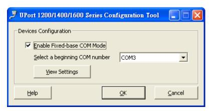
Fixed-base COM Mode" allows users to specify which COM number will be assigned first. In addition, COM numbers are assigned sequentially, and are not tied to specific UPort converters. For example, assume that you have set COM10 as the first COM number that will be assigned. If UPort D1 is plugged into your computer first, your computer will assign COM10 and COM11 to the UPort's serial ports. When UPort D2 is plugged in, the computer will assign COM numbers COM12 and COM13.
