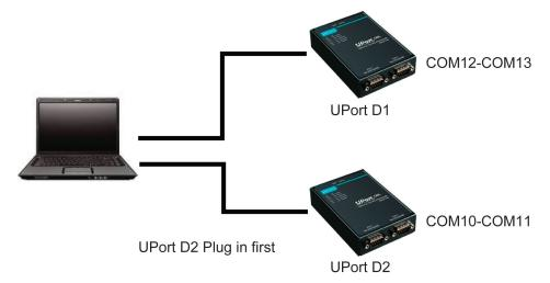
When "Fixed-base COM Mode" is enabled for the first time, all COM port numbers and serial port parameters will be reset to their default values. You can then set the COM numbers and configuration parameters to the values needed for your application.
