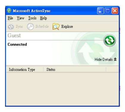
3. Click on the "**Explore**" button in the ActiveSync window, and then copy the UPort\_COM\_v1.0\_Setup.cab (Win CE 6.0) or UPort\_COM\_v1.1\_Setup.cab (Win CE 5.0) file to the "Mobile/Target Device".
