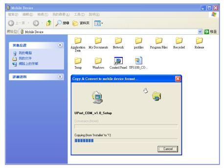
4. Double click on the CAB file (UPort\_COM\_v1.0\_Setup.cab (Win CE 6.0) or UPort\_COM\_v1.1\_Setup.cab (Win CE 5.0)) to start installing the UPort 1200/1400/1600 Series WinCE driver. After installing the driver, plug the UPort 1200/1400/1600 Series USB Serial device into the WinCE device's USB port. The driver will be loaded automatically, after which the UPort 1200/1400/1600 will be ready to use.
