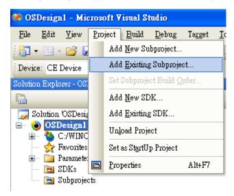
6. After the subproject is added, you may configure the "mxupce6.reg" registry file with the location [HKEY\_LOCAL\_MACHINE\Drivers\USB\ClientDrivers\MXU\_PORT].
