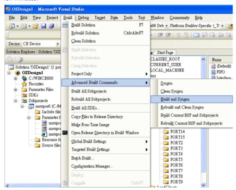
8. After building sysgen, select "**Build**" and "**Make Run-Time Image**" to create the WinCE OS image. Finally, copy your image file to the target Host.
