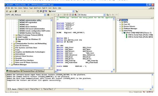
3. Right-click on the driver "USB to Serial Adapters (Prefix COM)" or "USB to Serial Adapters (Prefix MXU)" and then choose "Add to OS Design." After adding the driver, you will be able to find it in your workspace, after which you can start to build your OS and download it into a target.
