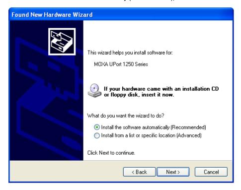
4. Wait while the installation wizard searches for the correct drivers. The next window that opens cautions you that although this software has not passed Windows logo testing, this driver has already been tested and shown that it can support the Windows operating system. Click **Continue Anyway** to proceed.
