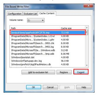
The most common usage of the Cache Content filter will likely be to permanently write content to the hard drive. To do this, select the file you wish to write to permanent memory and click on the **commit** button. This will delete the file from the cached overlay and replace the current file in permanent storage with the modified cache file.
