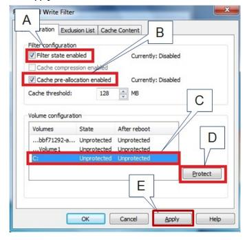
**NOTE** To minimize memory usage on the overlay cache, select **Cache compression enabled**. However, cache compression decreases performance when accessing protected volumes.
