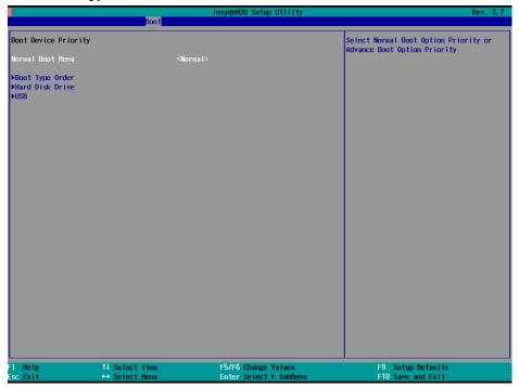
4. Select USB disk and then press "+" to move it to the first boot device position. Warning: An incorrect boot priority will lead to recovery failure.
