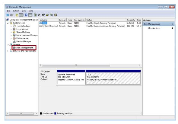
2. Insert the USB device that you want to save the system image to, in the USB port of the system. Click on **Disk Management** to view the size of the file system in **Disk 0** (sum of "**System Reserved**" and "**C:**").
