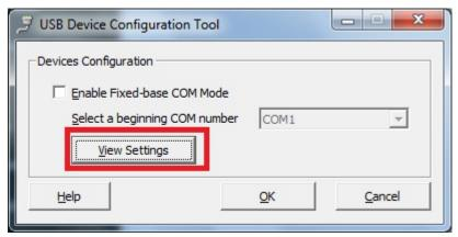
3. In View Settings, you can check which ports Windows is using for a MOXA Serial port; click OK to exit.
