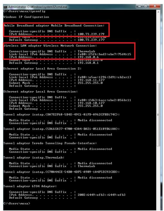
4. Windows 7 will choose the lowest Metric value for the connection interface if several routes are available for the same network destination and netmask. In this case, WiFi interface is the connection interface.
