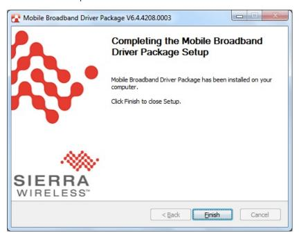
4. The system should locate the new hardware and install the driver automatically. Check the **Windows**Device Manager to verify.
