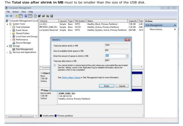
5. Make sure that the Total size after shrink in MB is smaller than the size of USB disk.
