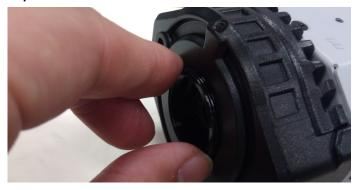
**NOTE** Be sure to loosen the screw affixing the lens holder in step 2 before trying to remove the lens holder. The lens holder may be too tight to loosen if the screw is not loosened first.
