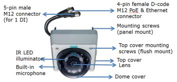
Mounting screw (panel mount): 4 nylock M4 screws (40 mm) are required to mount the VPort P16 on the wall or ceiling; the external length is about 20 mm after installation. The 4 mounting screws can work with the 4 sets of nut, gasket, and spring washer, or can be screwed directly into the screw holes.
