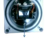
2 screws for fixing the lens in a horizontal position (5.5 kgf-cm)
