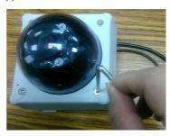
Step 2: Use the installation sticker for drilling the holes (gray color for panel mounting, green color for flush mounting).
